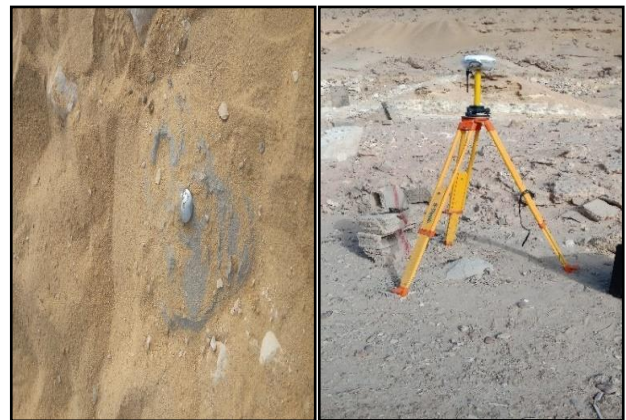
Figure 5: Control Point Fixation
