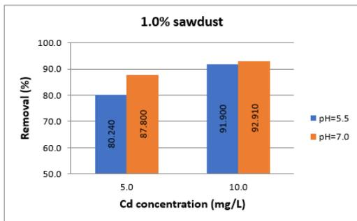
Fig. 8. Efficiency of Cd<sup>2+</sup> removal with 1.0 % sawdust at different pH values.
