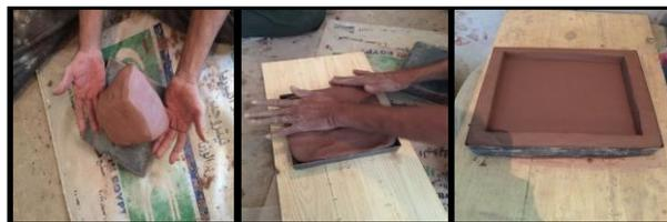
Photo (1): Forming the membranes filter shape
