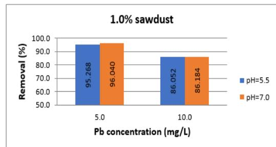
Fig. 5 Efficiency of Pb<sup>+2</sup> removal for the 1.0 % sawdust at different pH values.
