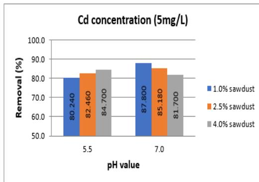
Fig. 3. Efficiency of Cd<sup>+2</sup> removal for the 5.0 mg/L-concentration at different ratios of sawdust.
