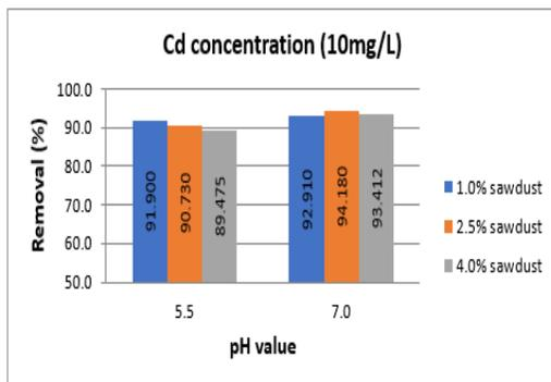
Fig. 4. Efficiency of Cd<sup>+2</sup> removal for the 10.0 mg/L-concentration at different ratios of sawdust.
