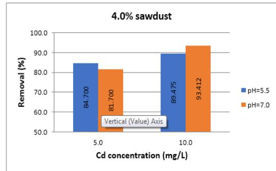
Fig. 10. Efficiency of Cd<sup>2+</sup> removal with 4.0 % sawdust at different pH values.
