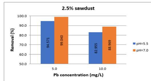
Fig. 6. Efficiency of Pb<sup>+2</sup> removal for 2.5 % sawdust at different pH values.
