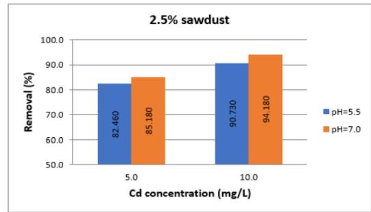
Fig. 9. Efficiency of Cd<sup>2+</sup> removal with 2.5 % sawdust at different pH values.
